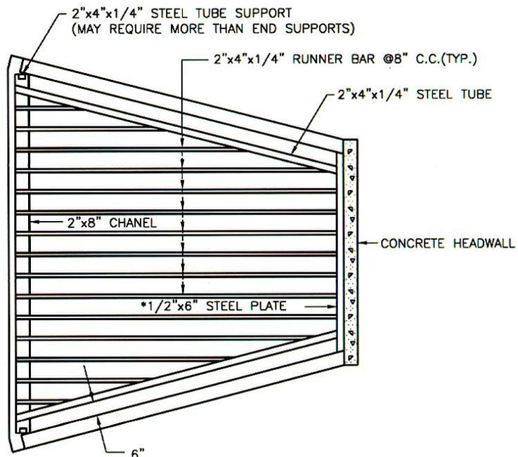
\* ATTACH WITH 5/8" RED HEAD WEDGE ANCHOR BOLTS.
